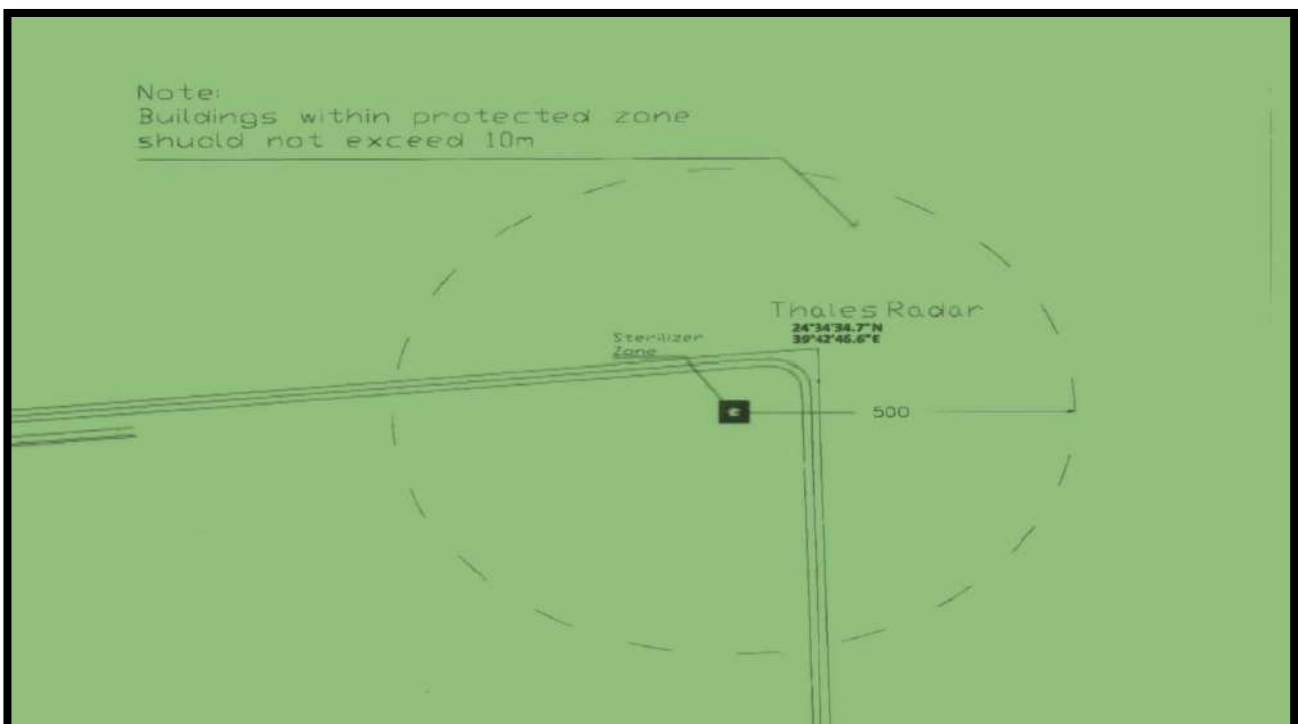
Figure 2 Radar Protection Zone – PMIA/OEMA
